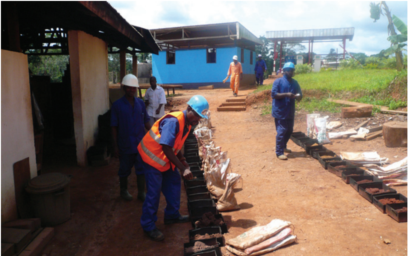
Sample preparation for assaying
